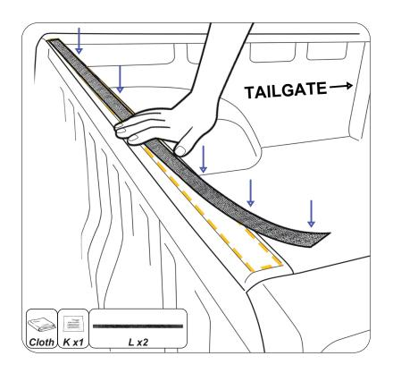
Clean any dust or dirt from top front edges of truck bed with clean cloth and then wipe down with surface cleaning wipe. Let the surface dry. Then apply Velcro strips with even firm pressure. Allow to cure for 24 hours for full bond strength.
